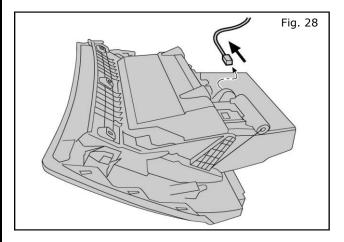
28. Carefully pull out the glovebox assembly. Remove the glovebox lamp. Fully remove the glovebox assembly and set aside.
