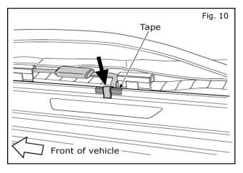
10. Cover the sheet metal edge under the wiring with a piece of protective tape. Remove all slack from the wiring at the plate end. Carefully bend the flat wire to fit tightly over the sheet metal edge.
