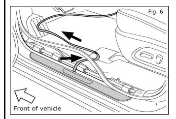
Place new Illuminated Kick Plate into position on the driver side door sill and feed the wiring through under the door welt.
