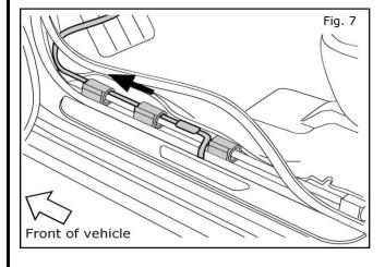
7. Feed the end of the wiring up through the existing harness clips towards the footwell.
