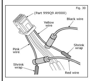
30. Using a posi-tap, connect the **Black** wire from the Kick Plate to the **Yellow** wire on the Accessory Connector Harness.
