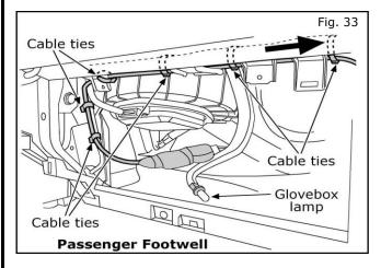
33. Route the **Red** and **Black** wires along the existing harness at the top of the glovebox cavity and out towards the A-pillar. Secure with cable ties as shown.
