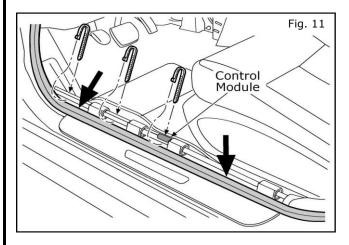
11. Press the door seal welt back down into position. Route the wires along the existing harness. Secure with cable ties as shown.
