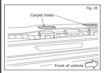
35. **Reinstall** the side trim panels on **both** sides of the vehicle along the bottom door seals from the seat to the footwell (see fig. 3).
