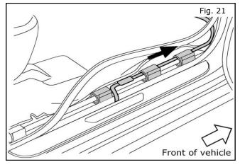
21. Feed the end of the wiring up through the existing harness clips towards the footwell.
