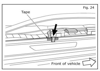
24. Cover the sheet metal edge under the wiring with a piece of protective tape. Remove all slack from the wiring at the plate end. Carefully bend the flat wire to fit tightly over the sheet metal edge.
