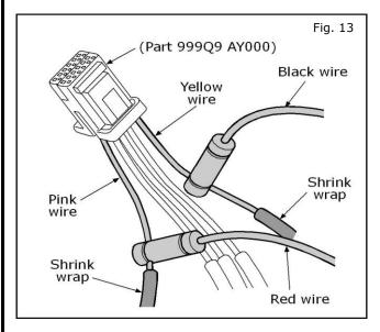
13. Using a posi-tap, connect the **Black** wire from the Kick Plate to the **Yellow** wire on the Accessory Connector Harness.
