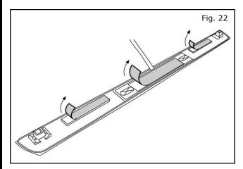
22. Carefully flip the Kick Plate over. Remove backing from three (3) adhesive strips located on the back of the Kick Plate.
