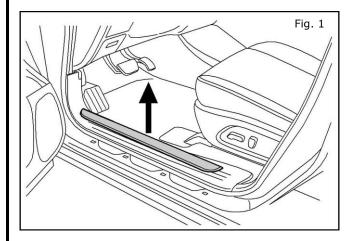
1. Use a trim stick to carefully pry off the existing kick plate from the driver side rocker area.
