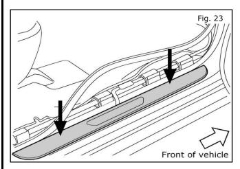
23. Carefully align Kick Plate with mounting holes and press firmly into position. Apply 15 lbs of downward pressure evenly along the Kick Plate for at least 30 seconds
