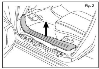
2. Use a trim stick to carefully pry off the trim panel along the bottom door seal from the seat to the footwell.
