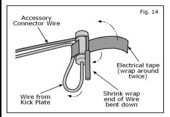
14. Follow this finishing procedure on all posi-taps. Leave a short length of wire extended past the posi-tap and bend down as shown. Use electrical tape to secure the extra wire against the posi-tap with at least two revolutions.
