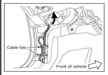
18. Route any excess wiring along the existing harness and up under the dash. Secure with cable ties.
