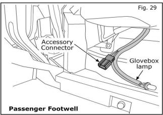
29. Locate the **passenger side** Accessory Connector plug. It will be located in the glovebox opening on the lamp harness.
