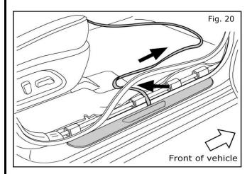
20. Place new Illuminated Kick Plate into position on the passenger side door sill and feed the wiring through under the door welt.
