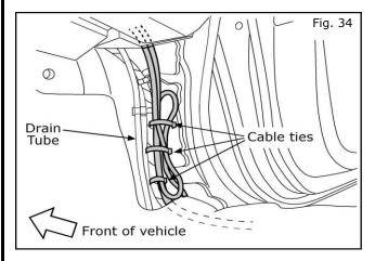
34. On the **passenger side**, route the wires along the existing harness and up under the dash. Secure any excess wire between the kick plate and the lighting control module with cable ties.
