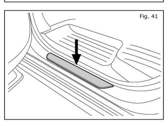
Note: Clean all mounting surfaces with alcohol wipe before final installation.
