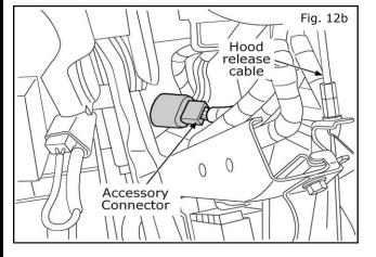
12b. This view shows the connector location looking up under the dash from below.
