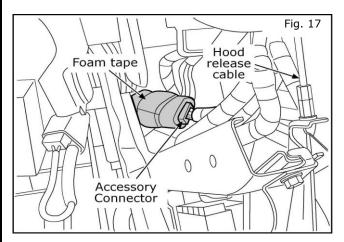
17. Wrap the Connectors in foam tape and position them back up inside the dash above the fuse block.
