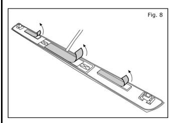
8. Carefully flip the driver Kick Plate over. Remove backing from three (3) adhesive strips located on the back of the Kick Plate.
