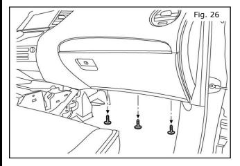
26. Remove three (3) phillips head screws from the underside of the glovebox.
