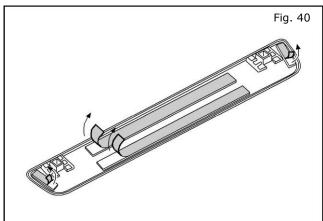
40. Remove backing from adhesive strips located on the back of the new Kick Plate.
