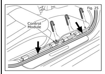
25. Press the door seal welt back down into position. Route the wires along the existing harness. Secure with cable ties as shown.
