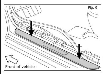
Carefully align Kick Plate with mounting holes and press firmly into position.
