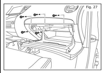
27. Open the glovebox door. Remove five (5) phillips head screws from inside the glovebox compartment.
